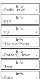
Cycle through Info menu by pressing the "D" button, select a particular option, then press the "MENU/SELECT" button to confirm. It will show the information on LCD.
